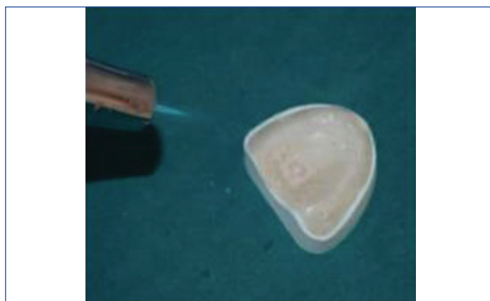
[Table/Fig-11]: Direct flaming of a denture base sample with butane torch.
