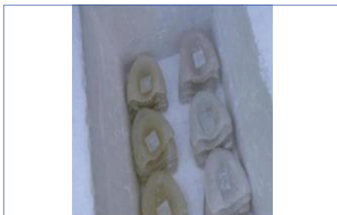
[Table/Fig-10]: Denture base sample in liquid nitrogen.
