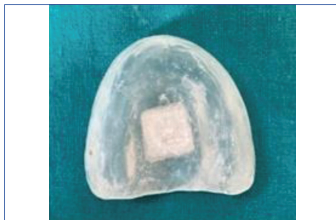
[Table/Fig-4]: Cold cure denture base sample with incorporated RFID tag.
