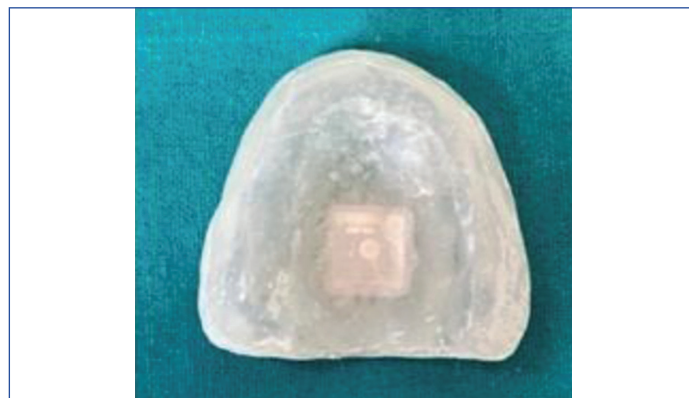
[Table/Fig-3]: Heat cure denture base sample with incorporated RFID tag.
